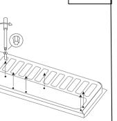
Remove OEM screws with Torx screw driver T15 "Save the Screws"
